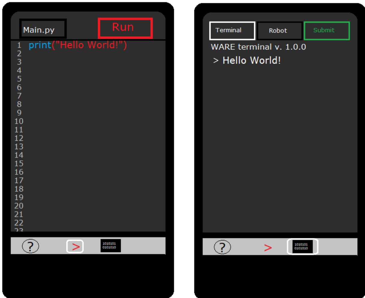
Figure 7.0.7: A potential display of the mobile display of the console and terminal. Users can swipe to the right and to the left to access both. In the terminal you can switch to the robot tab to see the robot visualization. This design would keep it as functional as it is on laptops and desktops - minus the upload file option.
